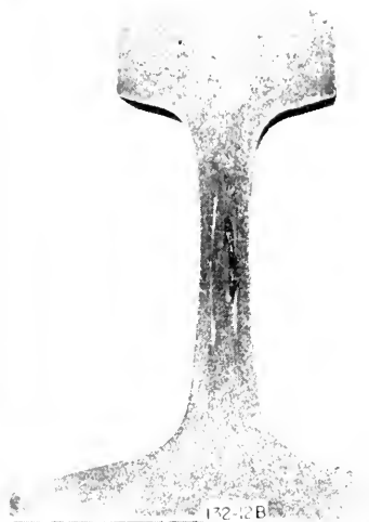
Fig. 9 (Investigation 132-12B)—Same cross section as in Fig. 8, after being macro-etched in a hot 50 percent aqueous solution of hydrochloric acid. The presence of a pipe and a non-metallic entrapment (slag) commonly associated with pipe can be noted in the web of this rail.
